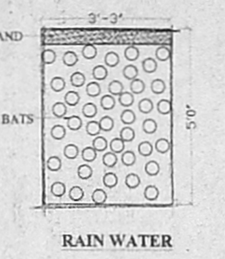
RAIN WATER PERCOLATION TRENCH
